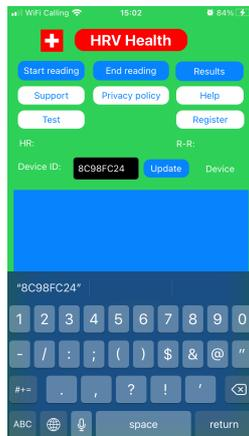
In the Device ID text field, enter your HRM device Id, and click the Update button. The app checks that the device Id is valid, and displays it in the box to the right of the Update button. If the number is incorrect, the field will display Invalid.
